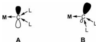
Scheme 2. Possible coordination modes of carbones with Lewis acids (M).
